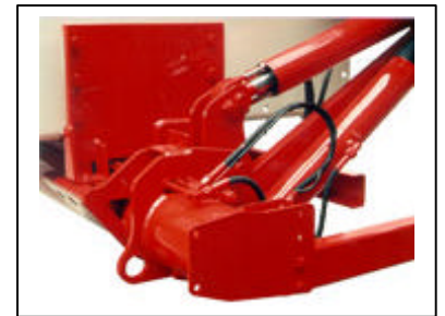
Retracted Hydraulic Cylinders are protected from damage caused by road debris.
